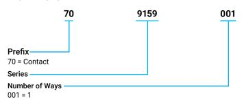
4XX 006 **Contact Description** 401 = PLUG - SMT 402 = Socket - SMT 411 = Plug - SMT - Locking **Packaging Options** 006 = Gold in Contact Area
