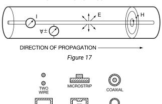
CROSS SECTIONAL CONFIGURATIONS OF VARIOUS TYPES OF GUIDING STRUCTURES
