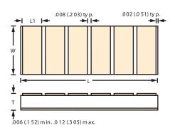
GA SERIES MULTIPLE PAD SLCs are ideal for circuits such as MMIC devices requiring multiple capacitance applications, i.e., bypassing and bias circuits. The GA Multicaps in the Selection Guide below are listed using KAVX's GA and K dielectrics, with a pad length of .015 (.380). However, other array designs are possible. Please consult factory.
