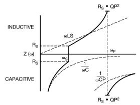
Figure 9. SLC Impedance Magnitude vs. Frequency
