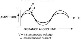
Pure traveling waves: V & I in the lossless case are in phase. V & I also reverse polarity every half wavelength.
