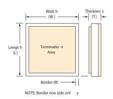
GP SERIES SINGLE RECESSED METALIZATION SLCs - have been designed to minimize potential shorting resulting from epoxy or solder attachments. Contact KAVX for further information.
