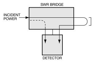
Figure 5. Return Loss Measurement: Establishing a Reference
